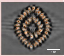
provides structural information on defects at the 2–3 Å scale. The authors suggest that their method is applicable to the atomic characterization of a wide range of nanostructures where strong electron channelling is absent, such as inorganic fullerenes.
